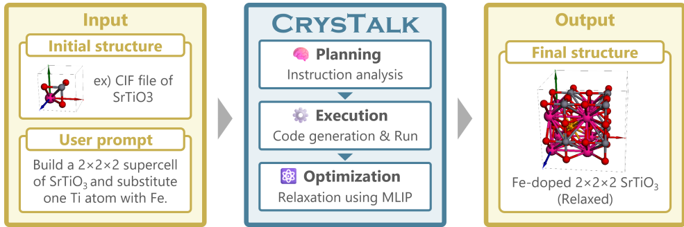
Figure 71: Workflow of CrysTalk. Given an input structure file and a user prompt, the agent performs planning, execution, and optional optimization to generate the final edited crystal structure.
